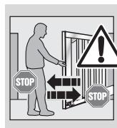
All persons using the gate system must be shown how to operate it properly and safely. Demonstrate and test the mechanical release as well as the safety return. To do this, halt the closing gate by grasping it with both hands. The gate system must initiate the safety return.
